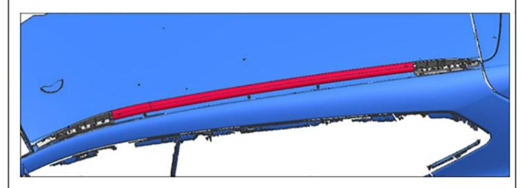
Step 9: Install the Front bottom cover and Rear bottom cover. Attention to Plastic clip match with aluminum bottoms and the direction of plastic clip is paralleled with bottoms. Mount the front and rear bottom covers on the roof rail. Remove 3M double-sided adhesive tape of the front bottom cover and push aluminum rod for clamping.
