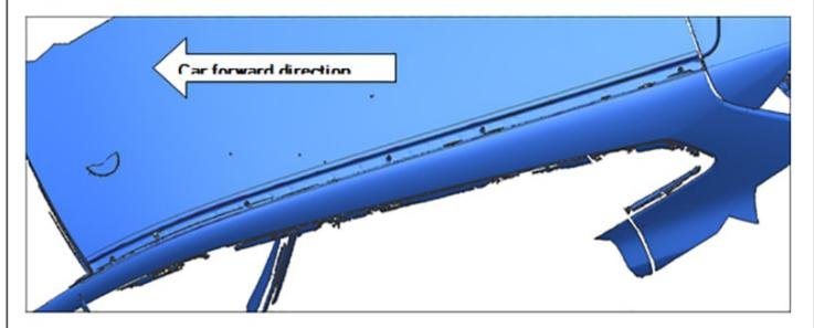
Step 3: Based on the front to remain 330mm, the mid to remain 925mm, cut the adhesive strip (if necessary) and restore installation.
