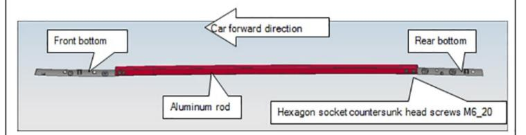
Step 8: Install the assembled roof rail on the car body with two Hexagon socket countersunk head screws M6\_20 to tighten up in the brackets.
