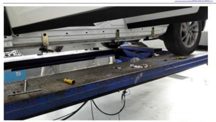
The distance for each Bracket with hanger against to the head skirt should be 34.5cm/105cm/159cm (as above photo).
