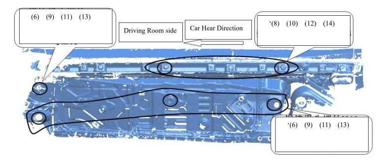
(2) Install the fixed bracket: first remove the original car guard plate, remove the corresponding screw and rubber plug of the original car, then place welding flat-head screws in the corresponding holes, and install the corresponding bracket into the car and lock it (the left and right installation methods are the
